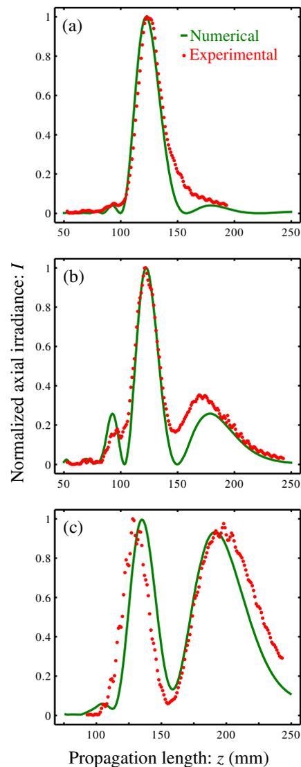
**Fig. 4.** Numerical simulation, continuous (green) lines and experimental results (dotted) red lines provided by the 3D printed THz lenses of Fig. 2: (a) Fresnel, (b) fractal, and (c) Fibonacci.
