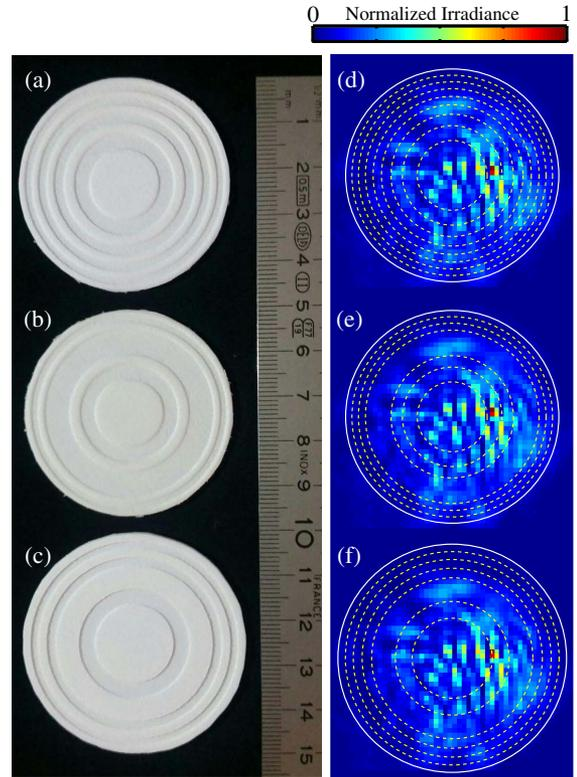
**Fig. 2.** Experimental (a) Fresnel, (b) fractal, and (c) Fibonacci models of 3D printed THz diffractive lenses made PA6. Map of the THz irradiance measured at the plane of the lens in the experimental setup represented in Fig. 3 (dotted lines represent the phase transitions) for (d) Fresnel, (e) fractal, and (f) Fibonacci lenses.
