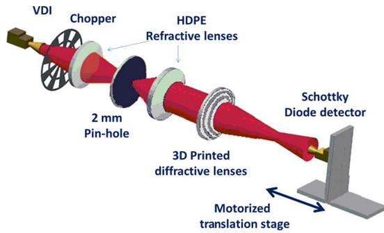
**Fig. 3.** Scheme of the optical setup used for axial PSF measurements.
