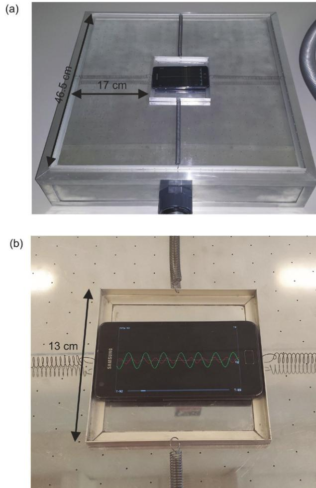
**Figure 2.** Experimental setup used for the experiments. In panel (a) a global view of the squared air table is shown. In panel (b), the detail of the smartphone and the squared tray holding it are shown. The dimensions of the air table and the tray are indicated on the picture.
