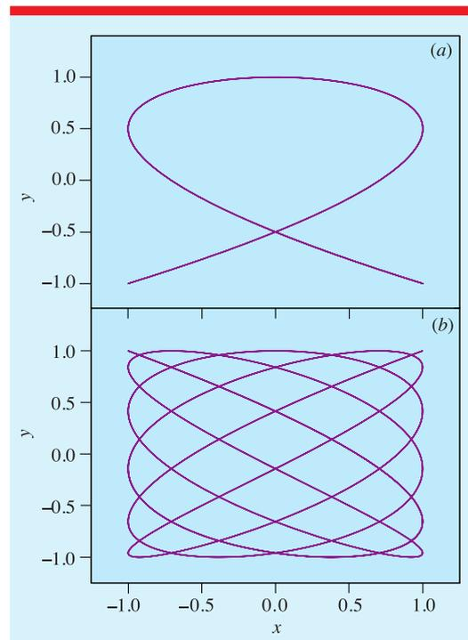
**Figure 6.** Theoretical Lissajous curves for  $T_x/T_y = 2/3$  in panel (a) and  $T_x/T_y = 8/11$  in panel (b). In both cases an amplitude of 1 arbitrary unit has been considered. The phase difference between  $x$  and  $y$  oscillations is 0 degrees.
