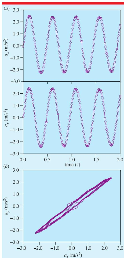
**Figure 3.** Results for Experiment 1 of (a) acceleration versus time on the  $x$ - and  $y$ -axes and (b) the corresponding Lissajous curve from  $a_y = f(a_x)$ .
