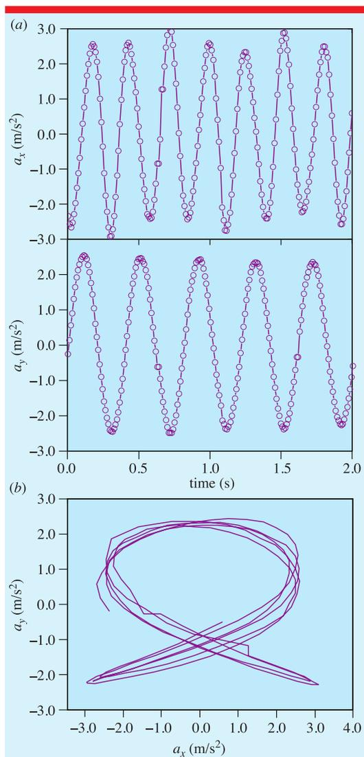
**Figure 4.** Results for Experiment 2 of the acceleration versus time on the  $x$ - and  $y$ -axes are shown in panel (a), and the Lissajous curve from  $a_y = f(a_x)$  in panel (b).
