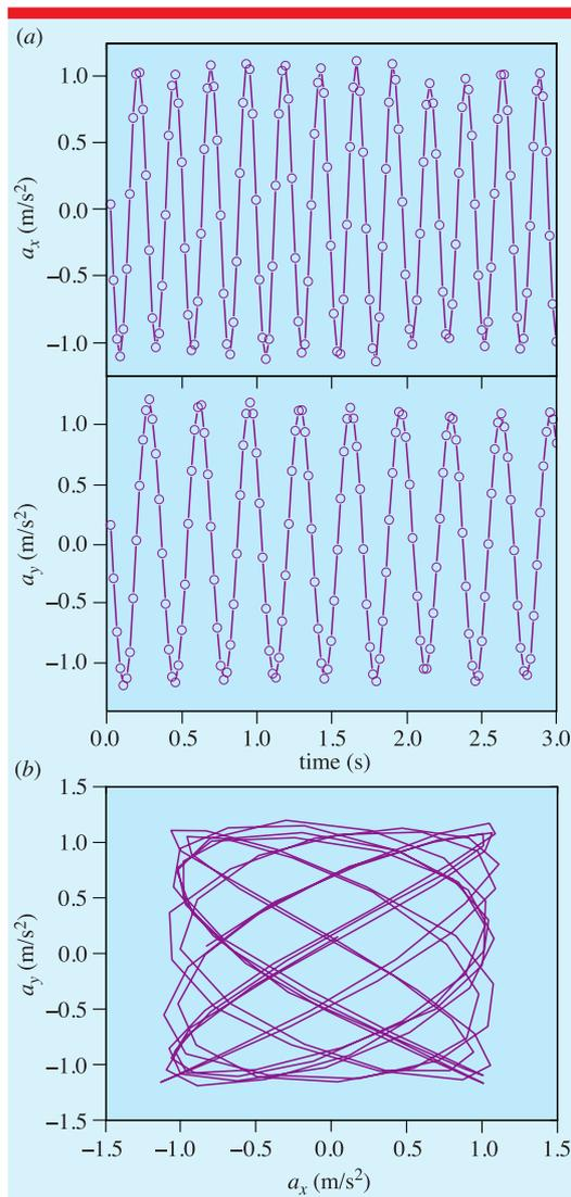
**Figure 5.** Results for Experiment 3 of the acceleration versus time on the  $x$ - and  $y$ - axes are shown in panel (a), and the Lissajous curve from  $a_y = f(a_x)$  in panel (b).
