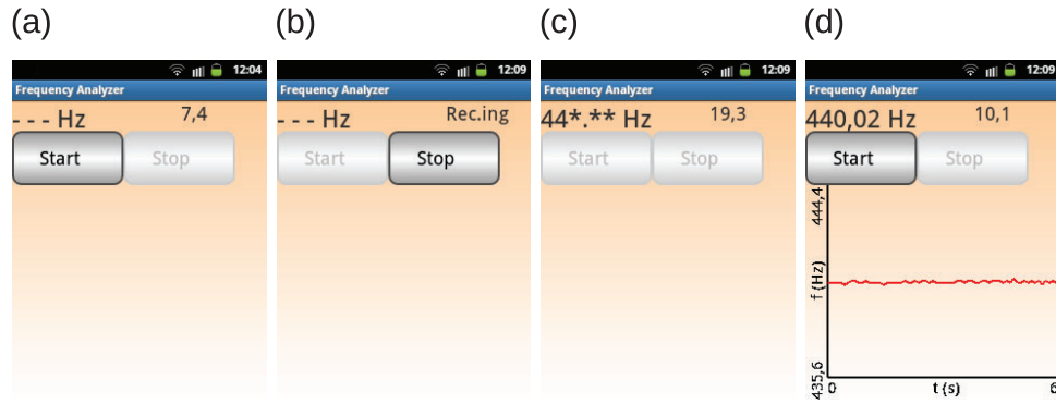
Figure 1 Snapshots of the Frequency Analyzer application, (a) at the start-up of the application, (b) in the process of recording data, (c) in the process of making calculations, and (d) result for one of the measurements. [Color figure can be viewed in the online issue, which is available at wileyonlinelibrary ].
