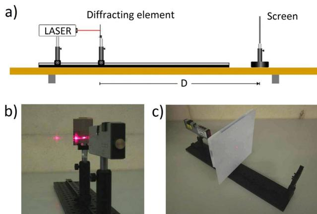
Fig. 1. (a) Schematic representation of the experimental set up, (b) device used to obtain the transmission diffraction pattern, and (c) device used to obtain the reflection diffraction patterns.
