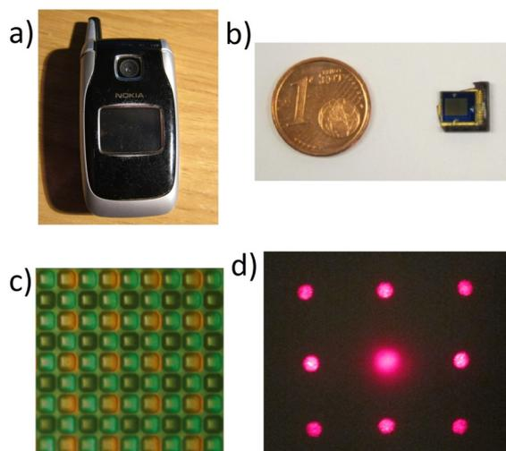
Fig. 2. (a) General view of the Nokia 6102 mobile phone, (b) photograph of the CCD sensor in comparison to a one (euro) cent coin, (c) the microscope image of the sensor, and (d) the central area of the reflection diffraction pattern.
