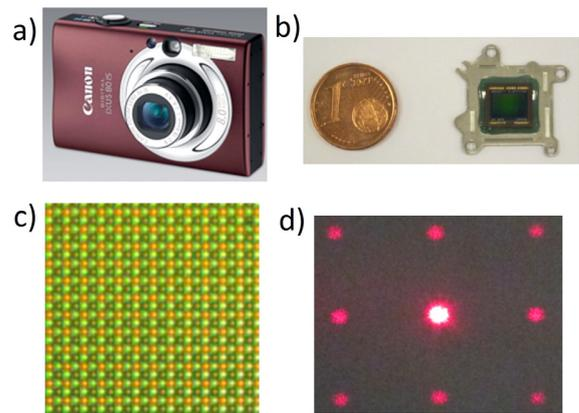
Fig. 3. (a) General view of the digital camera Canon Ixus 80 IS, (b) photograph of the CCD sensor in comparison to a one (euro) cent coin, (c) the microscope image of the sensor, and (d) the central area of the reflection diffraction pattern.
