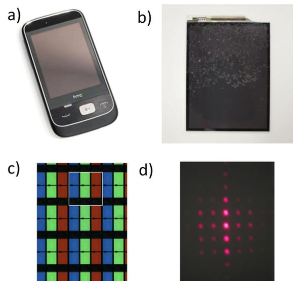
Fig. 4. (a) General view of the LCD screen of the HTC smartphone, (b) photograph of the screen panel, (c) its microscope image, and (d) the central area of the transmission diffraction pattern.
