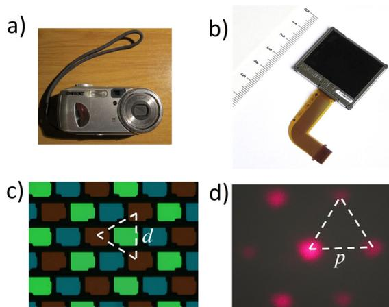
Fig. 5. (a) General view of the Sony DSC P73 digital camera, (b) photograph of the LCD screen, (c) its microscope image, and (d) the central area of the transmission diffraction pattern.
