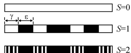
Fig. 1. Construction of a 1D fractal binary structure with the following parameters: N=4 , S=2 . \gamma is the scale factor and \varepsilon is the lacunarity.
