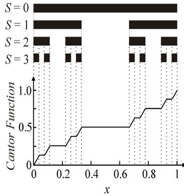
Fig. 1. Triadic Cantor set for  $S = 1$ ,  $S = 2$ , and  $S = 3$ . The structure for  $S = 0$  is the initiator and the one corresponding to  $S = 1$  is the generator. The Cantor function or Devil's staircase,  $F_S(x)$ , is shown under the corresponding Cantor set for  $S = 3$ .
