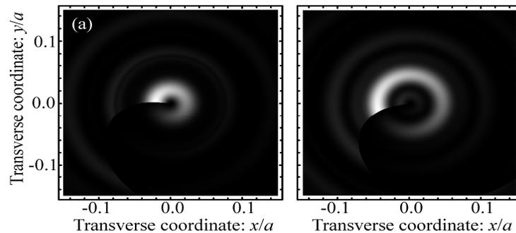
Fig. 4. Transverse field maps (as the product of the irradiance times phase) at (a)  $u = 9$  and (b)  $u = 9.8$  computed for the lens in Fig. 1(b) with  $m = 1$ . The animations Fig. 4a.avi ([Media 1](#), 1.62 MB) and Fig. 4b.avi ([Media 2](#), 2.18 MB) show the evolution of the vortices as they propagate along the optical axis.
