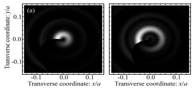
Fig. 4. Transverse field maps (as the product of the irradiance times phase) at (a) u = 9 and (b) u = 9.8 computed for the lens in Fig. 1(b) with m = 1. The animations Fig. 4a.avi (Media 1, 1.62 MB) and Fig. 4b.avi (Media 2, 2.18 MB) show the evolution of the vortices as they propagate along the optical axis.
