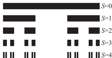
Fig. 1. Triadic Cantor set for the first levels of growth, S . The structure for S = 0 is the initiator and the one corresponding to S = 1 is the generator. Black regions correspond to the grooves etched in the fractal metallic grating (see Fig. 2)
