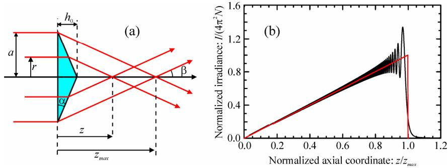
Fig. 1. (a) On-axis irradiance produced by a thin CL. The transverse radius of this axicon is  $a$ ,  $h_0$  is the height, and  $\alpha$  is the base angle. (b) Normalized axial irradiances given by a conventional CL for  $N=700$ , and the color lines correspond to a focusing geometry of an ideally infinite Fresnel number.
