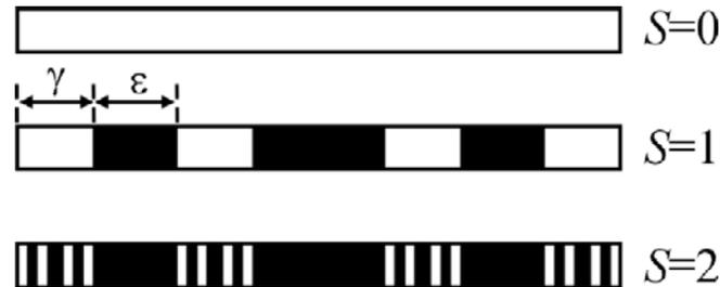
**Figure 6.** Schemes for the generation of the FZP binary function  $q(\xi)$  for  $N=4$  up to  $S=2$ .  $\gamma$  is the scale factor and  $\varepsilon$  is the parameter that characterizes the lacunarity.
