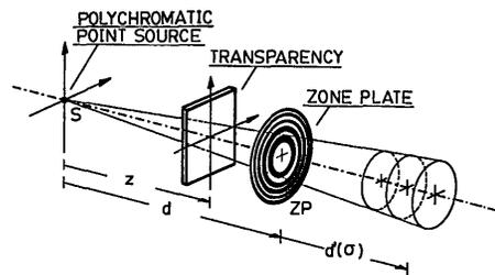
Fig. 2. Fourier-transforming properties of a blazed ZP under polychromatic spherical-wave illumination.
