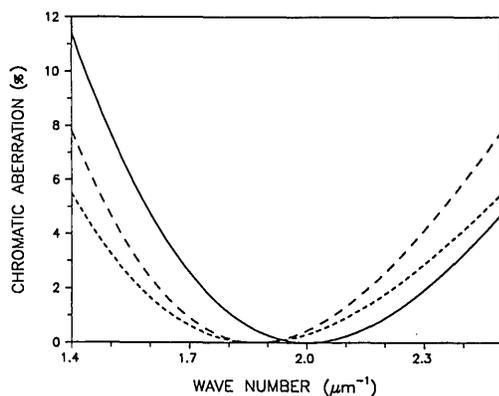
Fig. 4. Plot of the geometrical residual CA of the optical Fourier transformer in Fig. 3. Solid curve,  $\alpha = 1$  and  $\sigma_0 = 2 \mu\text{m}^{-1}$ ; long-dashed curve,  $\alpha = 1$  and  $\sigma_0 = 1.87 \mu\text{m}^{-1}$ ; short-dashed curve,  $\alpha = 0.3$  and  $\sigma_0 = 1.87 \mu\text{m}^{-1}$ .
