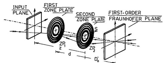
Fig. 3. All-diffractive achromatic Fourier transformer.
